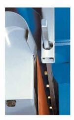
Each working unit motor is equipped with a **disk brake** to allow the machine to stop in a few seconds in case of emergency.
