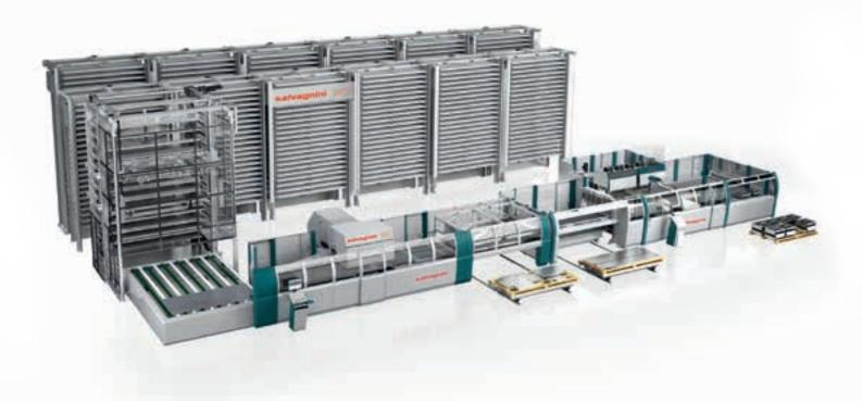
Salvagnini manufacturing lights out systems have the MV tray store as a hub. Thanks to Salvagnini's proprietary software the material is scheduled and sequenced through the punching, shearing, laser cutting and bending operations in a totally automated and integrated production environment.
