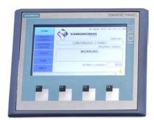
The parameters of ram position (distance table-ram), speed, electronic cams, mould protection device and countdown counter, can be easily stored through a software that permit several configurations, having a capacity of almost 200 Tool Programs. When recalling a Tool Program, the press automatically and simultaneously make all the set-up in a very short time. It is also possible to memorize Tool Programs in USB-key.
