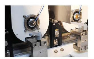
The "R" and "V" units are extractable to facilitate brush tool replacement and maintenance operations, they are designed to operate with standard, low-cost, brush cups as well as custom-made brushes for special applications.
