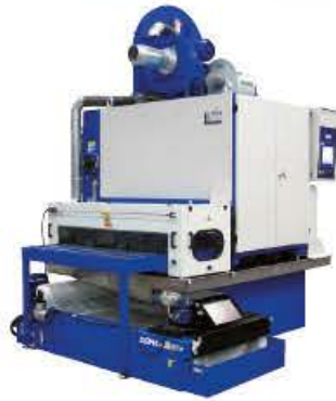
The dust generated by the working process is removed by a flow of water coolant.
