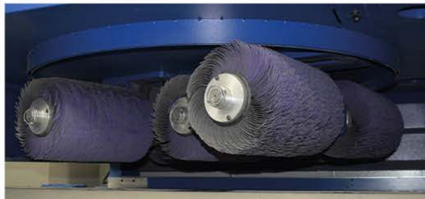
"RBC" Unit Rotary brush head carousel Rotating unit on vertical axis equipped with 8 counter-rotating \varnothing 350 mm brushes, mounted on horizontal axis
