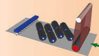
MD7 CBV • Deburring -Finishing • Edge Rounding • Oxide skin removal
