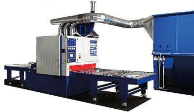
The dust generated by the working process is removed by an air flow.
