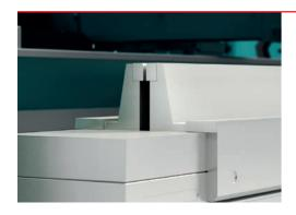
The MVM option, the variable opening die which is an alternative to ATA.L, automatically adapts the opening of the V on the basis of the program and allows materials with different thicknesses and/ or bending radii to be bent. It does not require manual die set-up, increasing the productivity and flexibility of the press brake.
