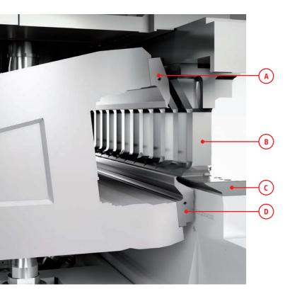
The upper and lower blades (A, D) are the two tools featuring interpolated controlled movement and responsible for bending.
