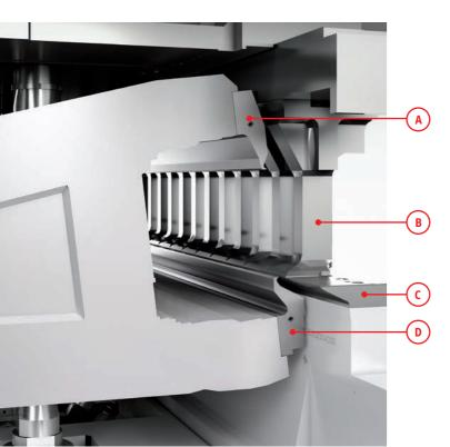
**The upper and lower blades (A, D)** are the two tools that feature interpolated controlled movement and are responsible for bending.
