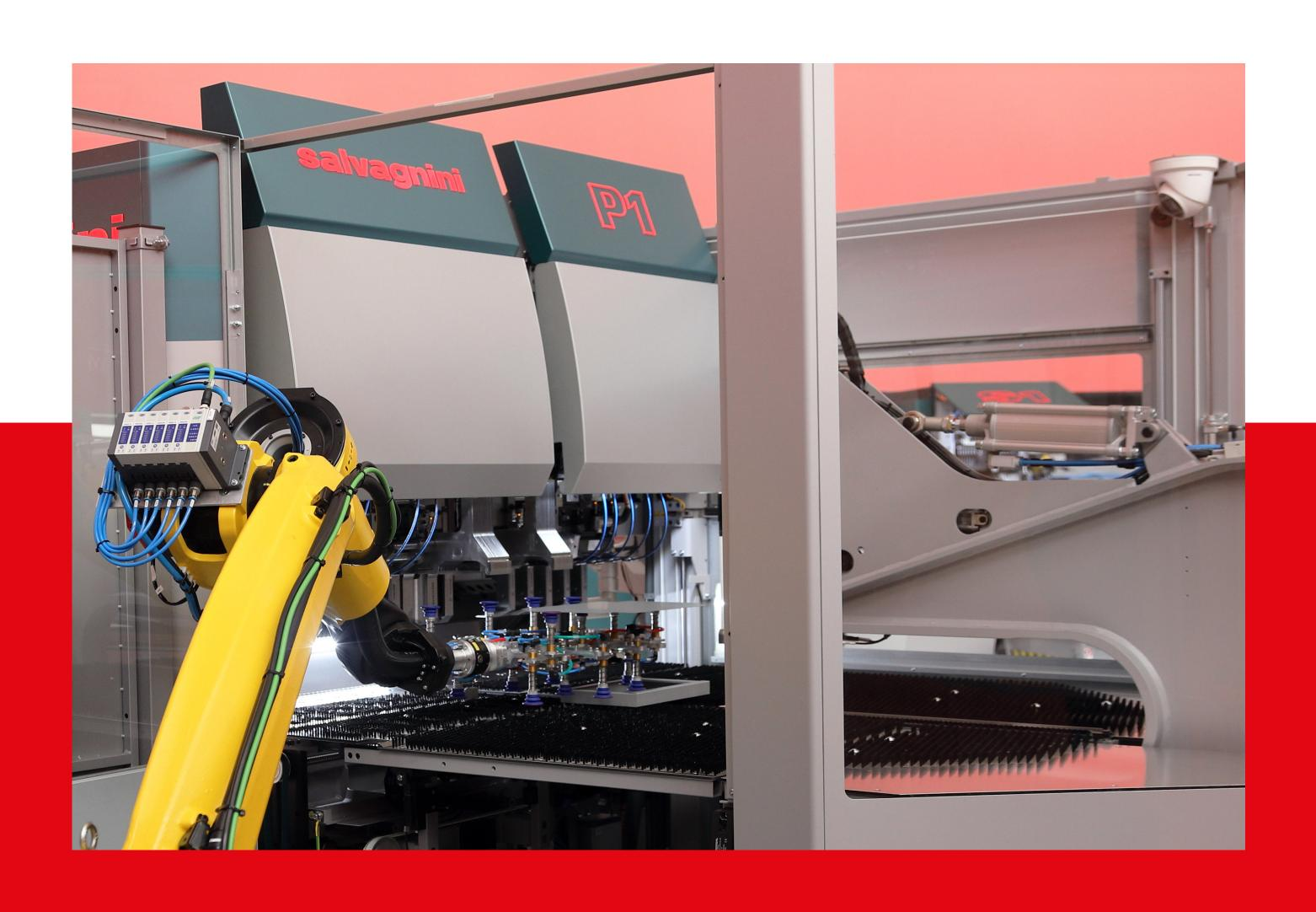
solutions with loading/unloading assistance only, or else more complex systems providing for automatic movement of the pallets or third-party integrations – for example with work centers for labeling, laser marking, riveting, welding, and corner forming."
