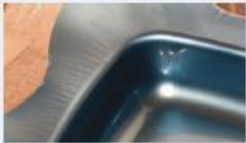
Wrinkles and buckles as a result of uncontrolled material flow during deep draw
